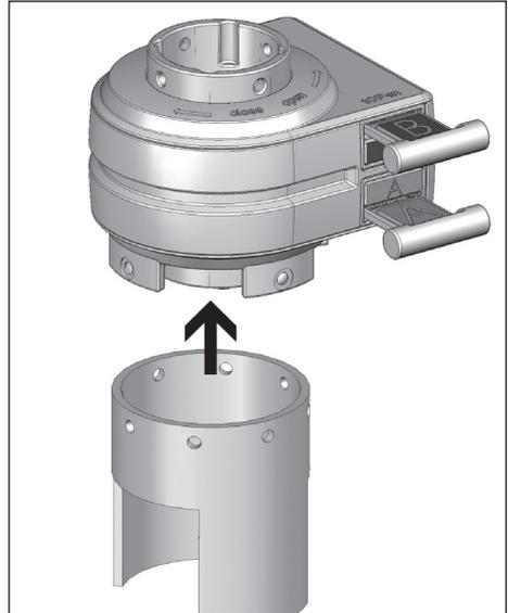
Fit the lever of the valve interlock on the shaft according to the valve position (parallel or crosswise to line). Tighten the lever with four threaded pins.
