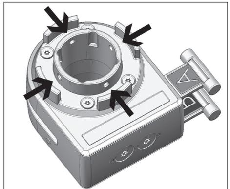
Align the valve interlock above the line so that the keys can be easily reached; four positions are possible.
