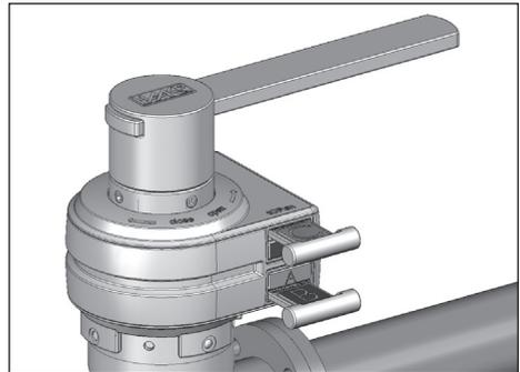
Turn the lever through 45° and by guiding the Allen key through the holes in the torque support, tighten the four already fitted threaded pins to secure the valve interlock at the adapter.
