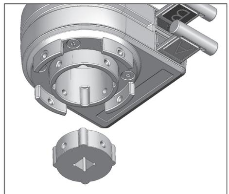
Fit the adapter in the valve interlock. By inserting the Allen key through the holes in the housing tighten the adapter with four threaded pins.
