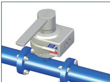
The valve is closed. The lower key **A** (red) can be removed. Upon removal of the key the valve is locked again and can no longer be operated. The upper key **B** (blue) remains trapped in the slot. The state of the valve (closed) is clearly visible from the vacant lower key slot.
